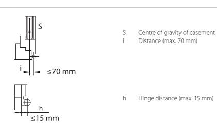
Only plastic window with steel reinforcement are approved.
